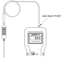
Figure 3. Probe Installation
